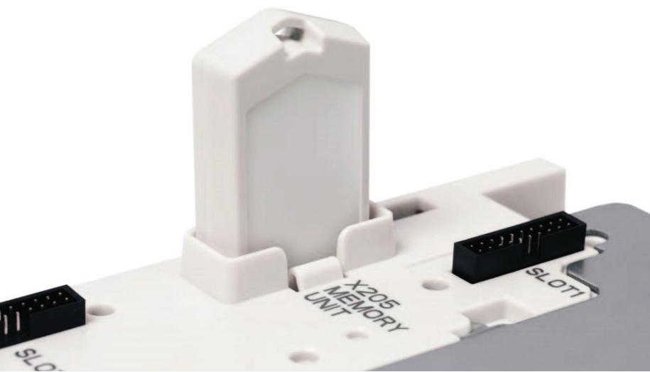
The removable memory unit stores the standard software that includes user settings, parameter settings and motor data and can easily be removed for maintenance, update or replacement purposes.
