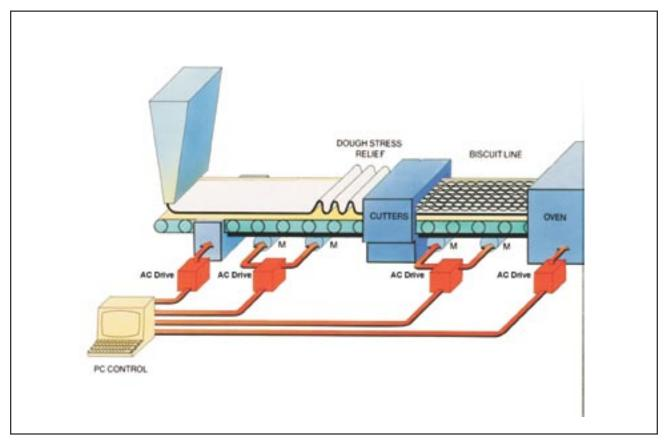
The ABB AC Drives' full digital control allows it to be interfaced as part of a modern process control system using a serial communications program. All alarm functions are displayed on a video screen and control of all Drives and motors is achieved from a single keyboard.
