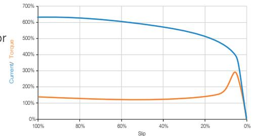
Figure 2: AC Induction Motor Current and Torque Curves
