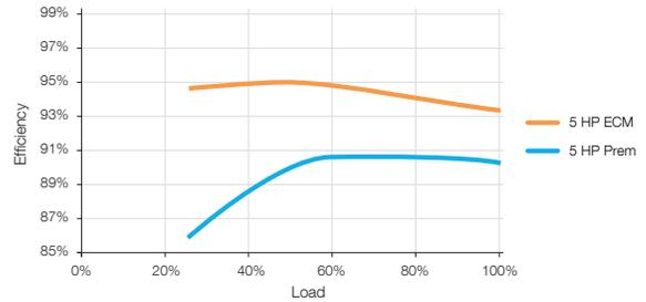
Figure 6: Efficiencies of 5 HP Induction Motor and ECM
