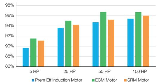
Figure 10: A Comparison of the Efficiencies of All Three Motors
