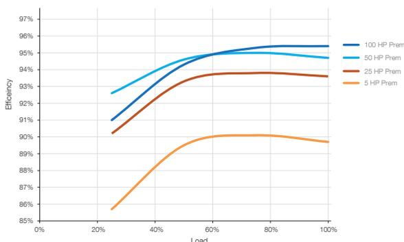
Figure 3: Efficiencies of Premium Efficiency Asynchronous AC Induction Motors
