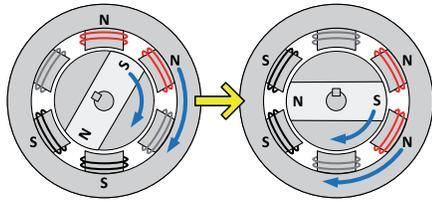
Figure 5: As the stator's magnetic field rotates, the magnets in the ECM's rotor follow it.
