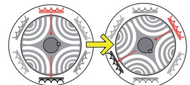
Figure 9: The regions of high magnetic permeability in the SynRM's rotor follow the stator's magnetic field.
