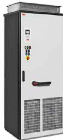
Our cabinet-built single drives are built to order, meeting your needs regardless of the technical challenges. The drive configuration includes a rectifier, DC link, inverter, fuses, line choke and a main switch, all built into a compact cabinet for easy assembly and commissioning.
